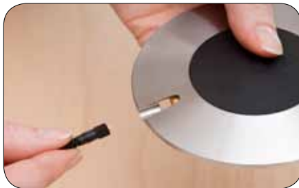
The MicroDot connector is assembled from the topside of the microphone.
