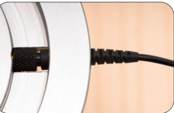
**Make sure the thread is firmly tightened.**
