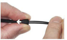
Before adjusting the frame size, you need to loosen the braided sleeving covering the cable. Remove the clothing clip, grab the bottom of the sleeving and pull it gently upwards, smoothing it up the entire length of the cable to make it loose at the top.
